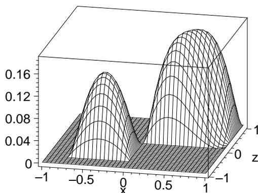
Figure 2: The higher-order part  $G_{hp}^B(x, z)$  of the discrete Green's function  $G_{hp}(x, z)$  for the Poisson equation with homogeneous mixed boundary conditions in  $\Omega = (-1, 1)$ , on a mesh with three elements  $[-1, -3/4]$ ,  $[-3/4, 0]$ , and  $[0, 1]$  of the polynomial degrees  $p_1=1$ ,  $p_2=2$ ,  $p_3=3$ .
