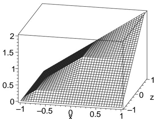
Figure 1: The lowest-order part  $G_{hp}^L(x, z)$  of the discrete Green's function  $G_{hp}(x, z)$  for the Poisson equation with homogeneous mixed boundary conditions in  $\Omega = (-1, 1)$  on a mesh with three elements  $[-1, -3/4]$ ,  $[-3/4, 0]$ , and  $[0, 1]$ .
