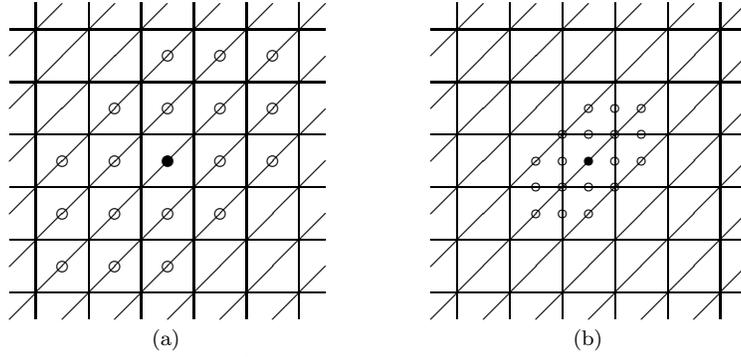
Figure 7: Sampling points for quadratic element
