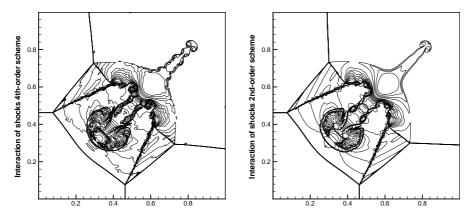
Figure 15: The density distribution for the fourth-order scheme and second-order scheme with  $\Delta x = \Delta y = 1/1000$  for the shock wave interactions.
