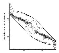
Figure 12: Density distribution and the local enlargement for the interaction of vortex sheets with different signs, with  $p_0 = 0.2$ .
