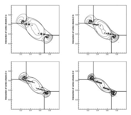
Figure 11: Density distributions for the interaction of vortex sheets with different signs, with  $p_0 = 1,0.75,0.5$  and 0.3.
