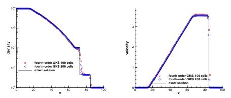
Figure 3: Large density ratio problem with density variation from 10000 to 1 starting from t = 1.2.
