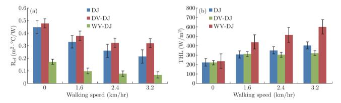
Fig. 3: Thermal resistance  $(R_{cf})$  and total heat loss (THL) of Dry jacket (DJ), wet vest and dry jacket (WV-DJ) and dry vest and dry jacket (DV-DJ) for various walking speeds
