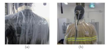
Fig. 2: Thermal manikin clothed with: (a) cooling vest and PVC membrane (A), and (b) firefighter's ensemble and PVC membrane (B)
