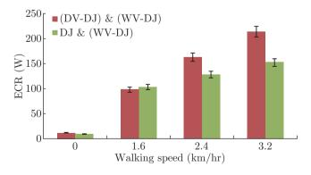
Fig. 4: Estimated cooling rates for wet vest-dry jacket (WV-DJ) and dry vest-dry jacket (DV-DJ) for various walking speeds (km/h)
