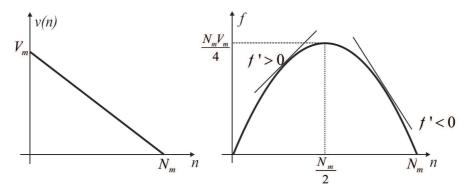
Figure 1: Curves in the Greenshield model for both the velocity v(n) (left) and the flux f(n) = nv(n) (right).
