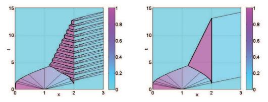
Figure 3: Left: Traffic through the traffic light where  $\alpha = 1/3$  is periodically stopped, and the queue is only partly cleared in each green light phase during a time of  $t \approx 14$  units. Right: Traffic through the roundabout where  $\beta = 1/3$  proceeds with a reduced flow, and the queue is cleared after the time of  $t \approx 14$  units.
