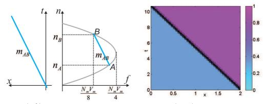
Figure 4: (Left) The flux diagram to determine the shock line. (Right) Contour plot of the computed traffic density on the upstream side of an intersection.
