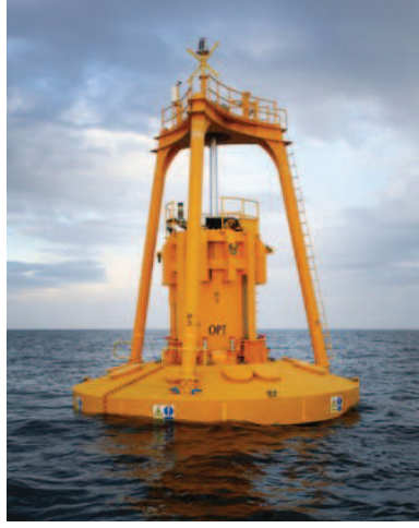
Figure 1: Deployed heaving buoy device PowerBuoy, at the northeast coast of Scotland. [25]
