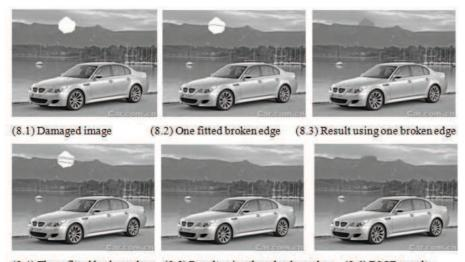
(8.4) Three fitted broken edges (8.5) Result using three broken edges (8.6) BSCB result. Figure 8: Repairing effects of different numbers of broken edges and comparison with BSCB result.
