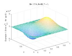
Figure 3: Error  $e_y = W - \partial u / \partial y$  at the mesh points for  $\alpha = 0.1$ .
