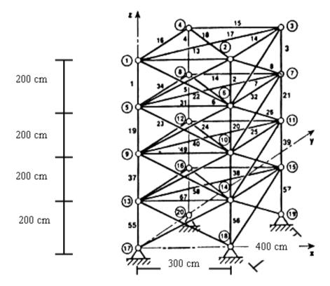
Figure 3: Space truss of Example 2.
