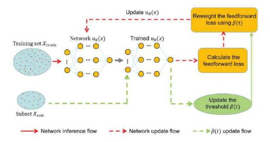
Figure 6: The proposed learning framework. A sub-training set  $X_{sub}$  is employed to update the threshold  $\beta(t)$  at the *t*-th iteration step. Then, the threshold  $\beta(t)$  is used to dynamically re-weight each training sample, especially lightening the importance of the samples close to the layer regions.
