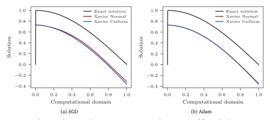
Figure 1: Predictions of PINN under various parameter initializations using SGD and Adam optimizers, respectively.
