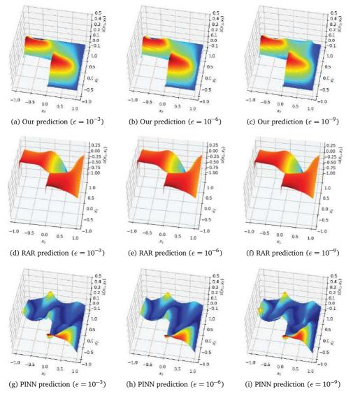
Figure 11: Comparison of RAR [23], PINN, and our approach for Eq. (5.5) with various diffusion coefficients on *L*-shaped domain.
