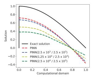
Figure 4: Predictions of PINN using a dense sampling in the layer domain, where 2500 points are sampled in the non-layer domain (0.1, 1), and 2500, 12500, 25000 points are sampled in (0, 0.1), respectively. For standard PINN, we apply a random sampling in (0, 1).
