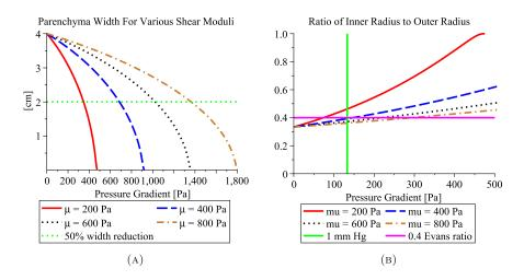
FIGURE 5. Incremental simulation of parenchyma width (A) and Evans ratio (B) as the total applied pressure gradient is increased in increments of 5 Pa. Note that 1 mm Hg = 133 Pa.
