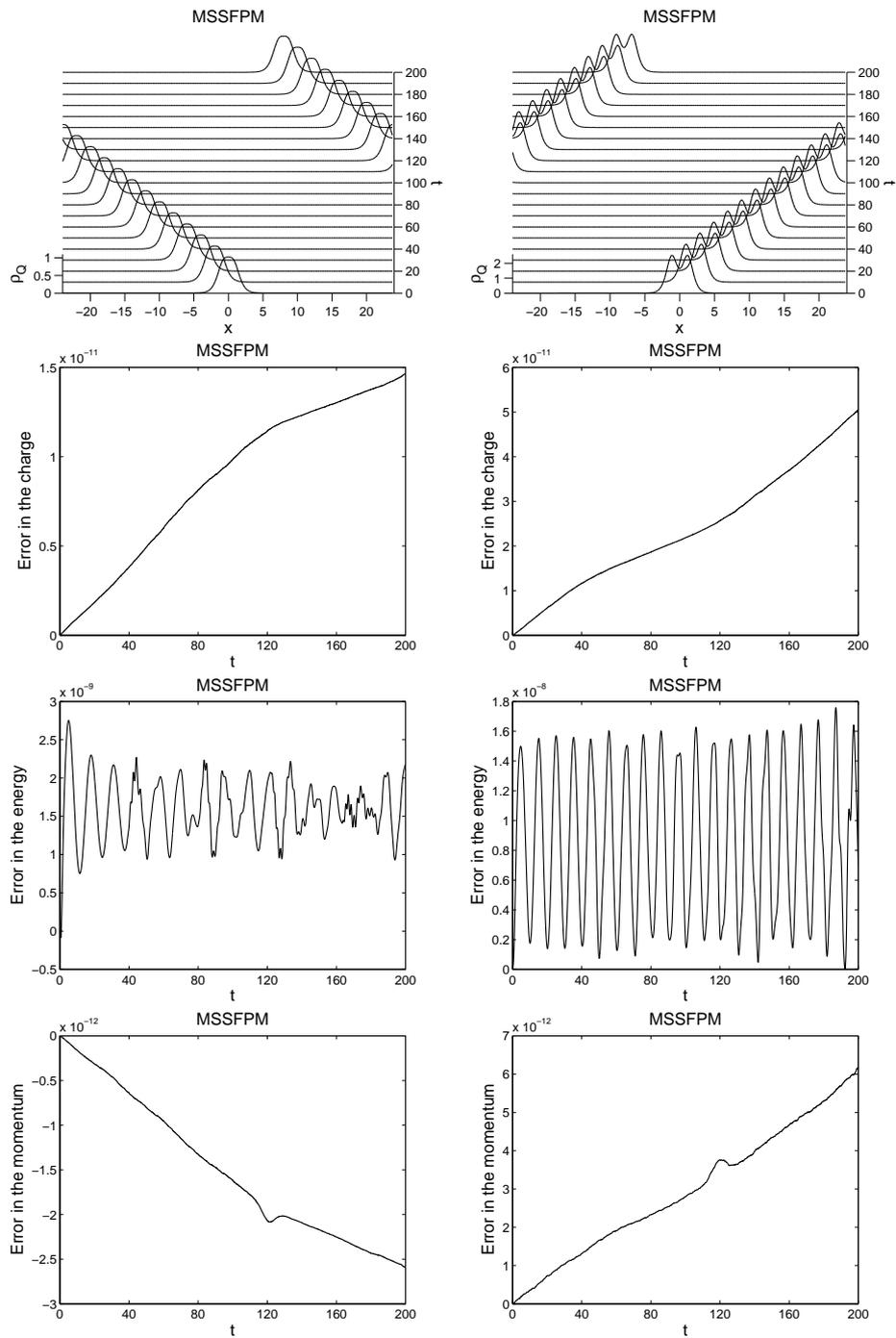
Figure 4: Propagation of one soliton of the NLD equation (1.3) and its corresponding errors obtained by MSSFPM with  $x_0=0$ ,  $[x_L, x_R]=[-24, 24]$ ,  $N=200$ ,  $\Delta t=0.01$ . Left:  $\Lambda=0.5$ ,  $v=-0.2$ , right:  $\Lambda=0.2$ ,  $v=0.2$ .
