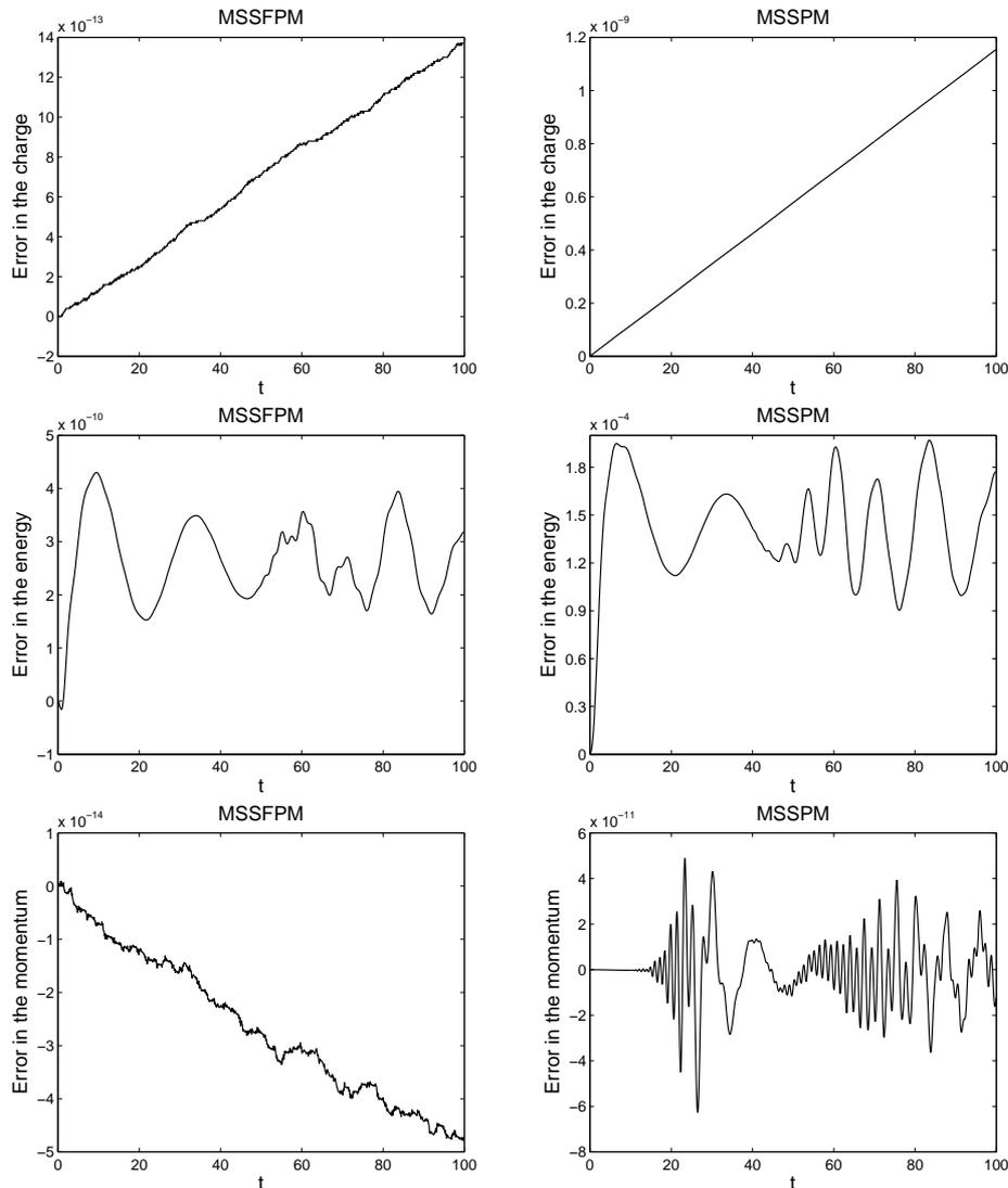
Figure 3: Corresponding errors in the discrete charge, energy and momentum obtained by the MSSFPM and the MSSPM.
