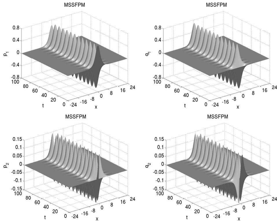
Figure 1: The four numerical solitary wave functions obtained by using MSSFPM with initial condition  $\Psi^{sw}(x,0)$ ,  $\Lambda = 0.75$ ,  $[x_L, x_R] = [-24, 24]$ ,  $N = 160$ ,  $\Delta t = 0.01$ .
