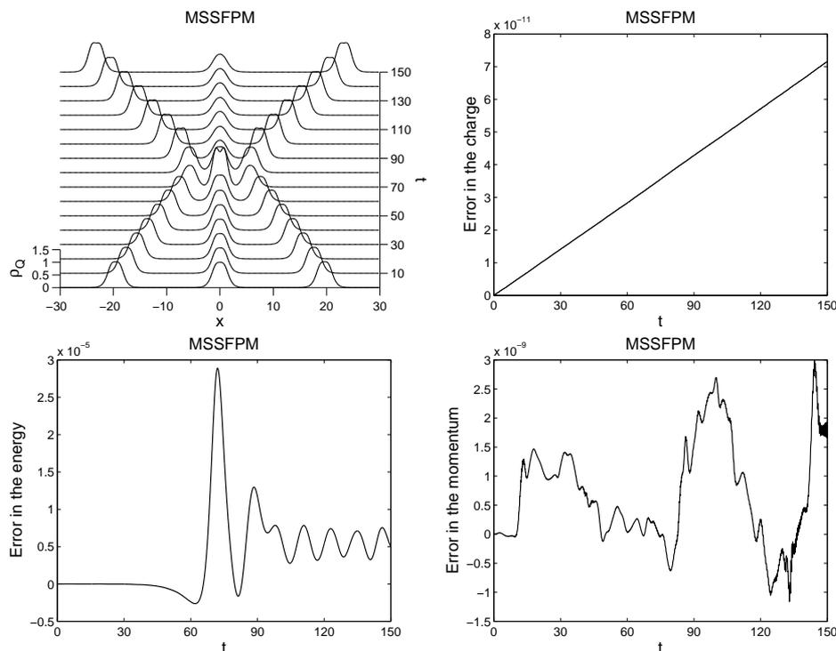
Figure 6: Interaction of three solitons of the NLD equation (1.3) and their corresponding errors obtained by MSSFPM with  $v_l = -v_r = 0.2$ ,  $v_m = 0.0$ ,  $x_r = -x_l = 20$ ,  $x_m = 0$ ,  $\Lambda_l = \Lambda_m = \Lambda_r = 0.5$ ,  $[x_L, x_R] = [-30, 30]$ ,  $N = 300$ ,  $\Delta t = 0.01$ .
