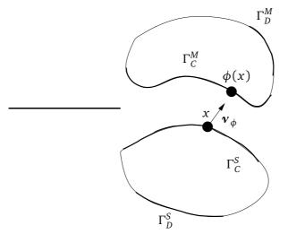
Figure 1: Two body contact problem and decomposition of the boundary.
