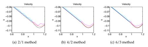
Figure 11: Grid convergence study. Close up view of the velocity at time 0.908 for h = 0.05 (fluid-cyan, solid-magenta), h = 0.025 (fluid-blue, solid-red). Reference solution shown in black.
