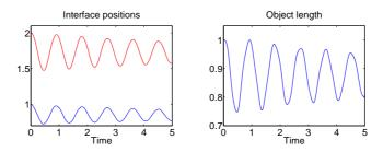
Figure 10: The position of the two fluid/solid interfaces as function of time (left) and the length of the rod as function of time (right). The 4/2 method with h=0.0125 was used.
