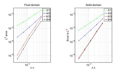
Figure 6: Errors in solution at time 0.45 in  $L^2$ -norm for the fluid domain (left) and solid domain (right). Summation by parts finite difference approximation of formal orders interior/boundary, 2/1 (green), 4/2 (blue), 6/3 (red) and 8/4 (black).
