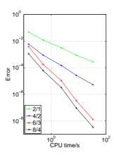
Figure 7:  $L^2$ -norm errors vs. CPU time. Summation by parts finite difference approximation of formal orders interior/boundary, 2/1 (green), 4/2 (blue), 6/3 (red) and 8/4 (black).
