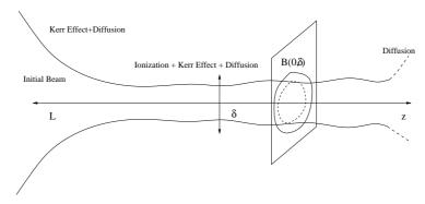
Figure 4: Single filament evolution.
