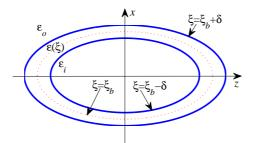
Figure 1: Schematic illustration of a three-layer dielectric model: The inner layer ( $\xi \leq \xi_b - \delta$ ) has a dielectric constant of  $\varepsilon_i$ , while the outer layer ( $\xi \geq \xi_b + \delta$ ) has a dielectric constant of  $\varepsilon_o$ . The intermediate translation layer ( $\xi_b - \delta < \xi < \xi_b + \delta$ ) assumes a continuous dielectric permittivity profile  $\varepsilon(\xi)$  that connects  $\varepsilon_i$  and  $\varepsilon_o$ .
