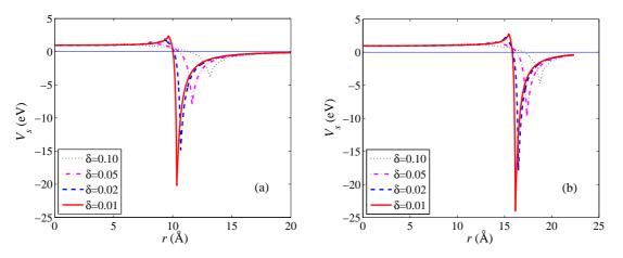
Figure 5: Self-polarization energy  $V_s$  of a prolate spheroidal QD as a function of r corresponding to the quasiharmonic model with  $\delta = 0.01, 0.02, 0.05$  and 0.1. (a) along a minor axis of the prolate spheroidal QD, and (b) along the ray pointing to the point (10, 0, 20).
