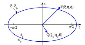
Figure 9: Schematic illustration of the step-like dielectric model: the dielectric constants of a prolate spheroid and the surrounding medium are  $\varepsilon_i$  and  $\varepsilon_o$ , respectively. The prolate spheroid, defined by the equation  $\xi = \xi_b$ , has an interfocal distance a. A point charge  $e_s$  is located at the point  $\mathbf{r}_s = (\xi_s, \eta_s, \phi_s = 0)$  in the *xz*-plane.
