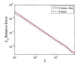
Figure 7:  $L_2$ -relative error in the self-polarization energy corresponding to the linear and the cosine-like models with  $\delta = 0.1$ , respectively, using the proposed numerical method with various L values.
