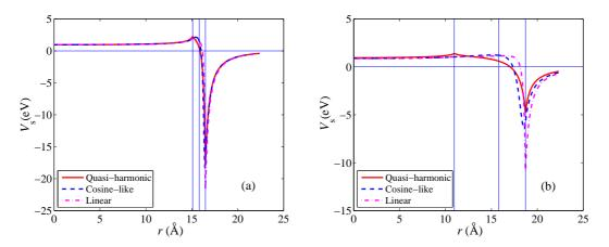
Figure 8: Self-polarization energy  $V_s$  as a function of r for several three-layer dielectric models with (a)  $\delta = 0.02$  and (b)  $\delta = 0.1$ , respectively. Solid line, the quasi-harmonic model with using the analytical solution; dashed and dot-dashed lines, the cosine-like and the linear models with using the proposed numerical method.
