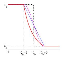
Figure 2: Illustration of several dielectric models for the translation layer between  $\xi_b - \delta$  and  $\xi_b + \delta$ , assuming  $\varepsilon_i > \varepsilon_o$ . Dot-dashed line, the step-like model; dotted line, the linear model; dashed line, the cosine-like model; and solid line, the quasi-harmonic model.
