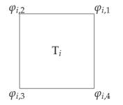
Figure 1: The rectangle element  $T_i$  and its four basis functions  $\{\varphi_{i,k}\}_{k=1}^4$ .
