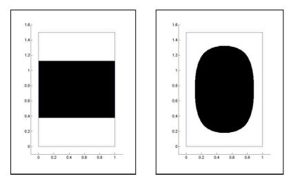
Figure 2: The profiles of the density distribution  $\rho$  in  $200 \times 300$  mesh grids.  $\Omega = [0,1] \times [0,1.5]$ ,  $\rho_1 = 1$  (in the subdomain of white color),  $\rho_2 = 2$  (in the black color) and  $\gamma_1 = \gamma_2 = 1/2$ . Left: the initial density distribution. Right: the density distribution at the stage of min $\lambda_1 = 7.3704$ .
