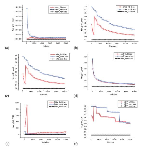
Figure 1: Results for flux\_g1k1, (a) mean, (b) relative error, (c) intrinsic error, (d) efficiency error (e) FOM, (f) VOV, versus number of histories.
