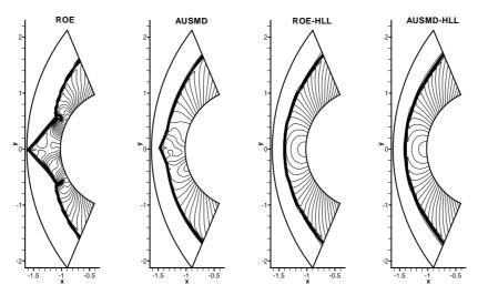
Figure 2: The contour of the pressure of Mach 20 hypersonic flow over a cylinder problem.
