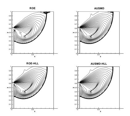
Figure 3: The contour of the density of diffraction of a supersonic shock moving over a  $90^\circ$  corner problem.
