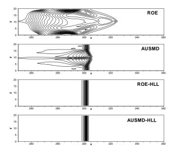
Figure 1: The contour of the density of odd-even grid perturbation problem.
