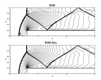
Figure 5: The contour of the density of forward facing step problem.
