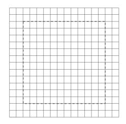
Figure 2: The structure of a grid block. Each block has  $12\times12$  interior cells bounded by dashed line and 2 guard cells on each side.
