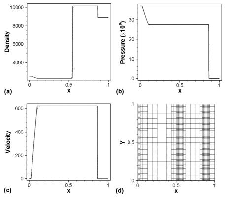
Figure 7: Results of a detonation product-copper Riemann problem at  $t=73\mu s$ .
