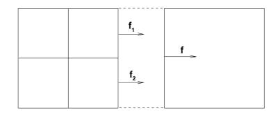
Figure 3: Flux conservation at a jump in refinement. In calculations,  $f = 0.5(f_1 + f_2)$ .
