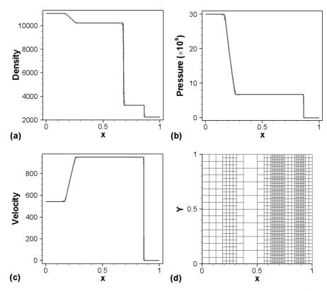
Figure 8: Results of the interaction between a shock in molybdenum and molybdenum-MORB interface at  $t = 120 \mu s$ .
