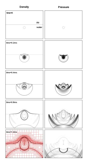
Figure 11: Schlieren images of density and pressure fields for the underwater explosion problem.
