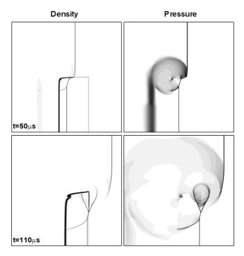
Figure 13: Schlieren images of density and pressure fields for shock interaction with a block of MORB.
