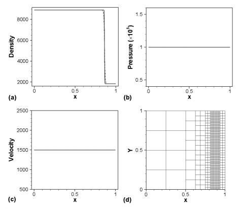
Figure 5: Cross-sectional results along y=0.5 for a copper-explosive interface advection problem  $t=240\mu s$ . The dash-dot lines are solution with AMR, while solid lines are solution with an uniform grid of 5000 cells. Frame (d) shows outlines of AMR blocks.
