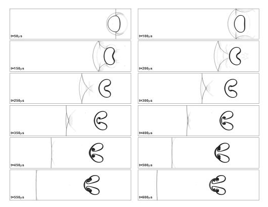
Figure 10: Schlieren images of density field for shock-helium bubble interaction.
