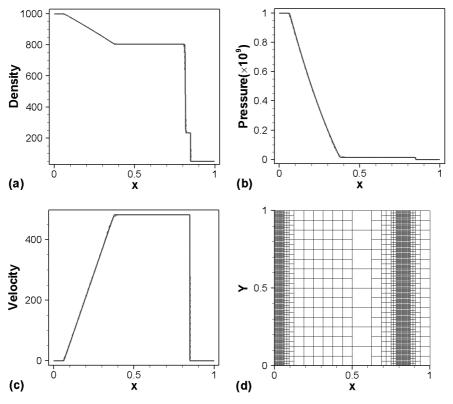
Figure 9: Results of a liquid-gas shock tube problem at  $t = 240 \mu s$ .
