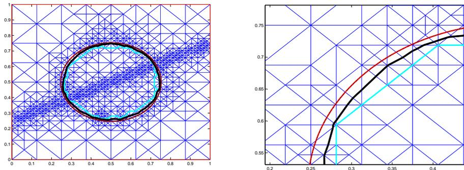
Fig. 5.1. Left: The red line depicts the boarder of the active set of the continuous solution, the black lines depict the boarder of the active set when using variational discretization with piecewise linear, continuous states, and the cyan line depicts the boarder of the active set obtained by using piecewise linear, continuous controls, Right: Zoom.
