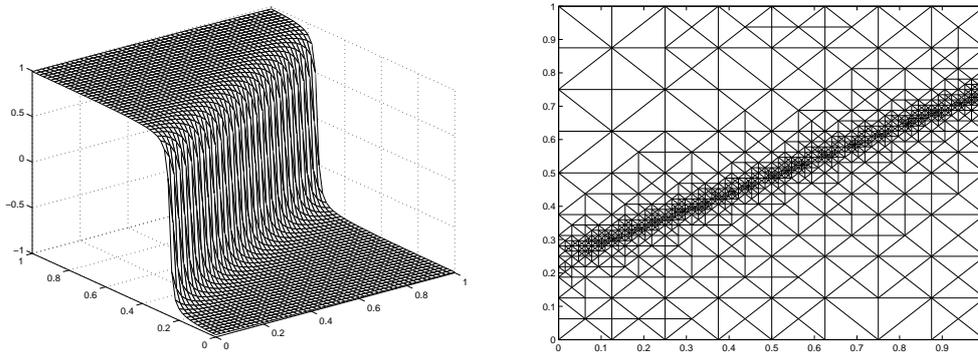
Fig. 5.1. Left: The surface of the state  $y$ ; Right: The adaptive mesh for the state  $y$ .
