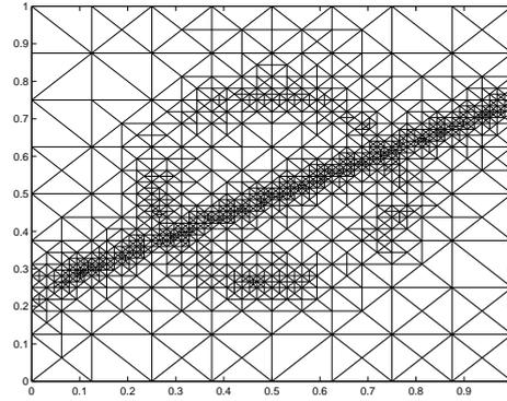
Fig. 5.4. The adaptive mesh for both  $y_h$  and  $p_h$ .Table 5.3: Comparison of the error of  $y, p$  and  $u$  on uniform and adaptive meshes.
