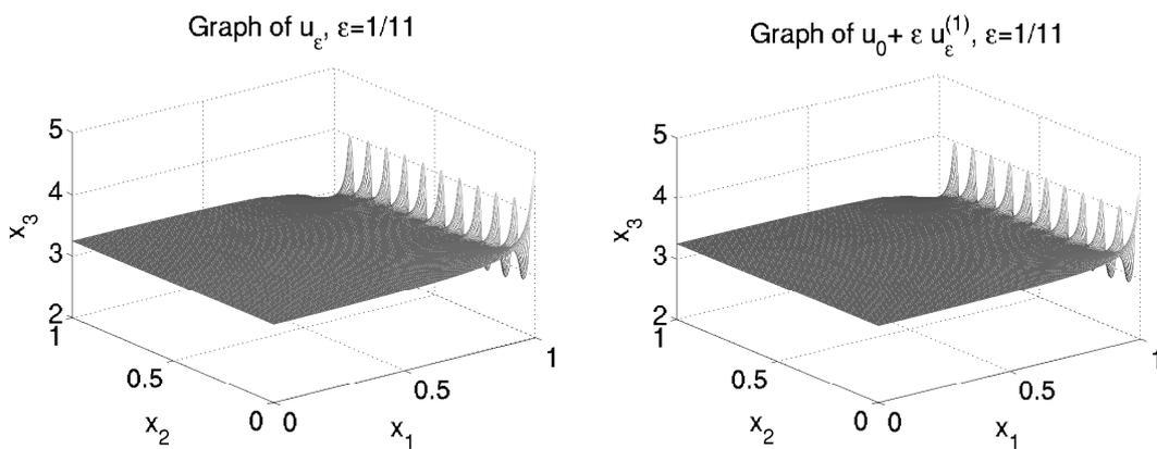
Fig. 5.6. Left: Brute force solution. Right: New approximation.  $\epsilon = 1/11$ .
