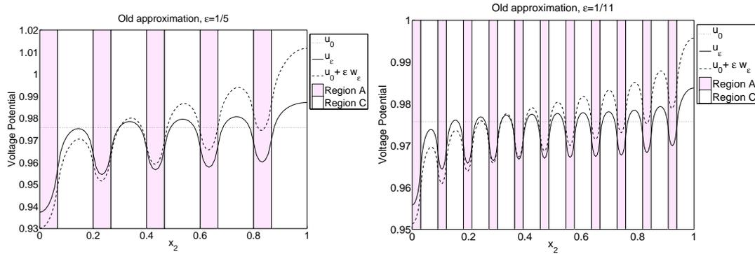
Fig. 5.1. Previous approximation and the brute force solution on the boundary  $\Gamma$ ,  $\epsilon = 1/5$ ,  $\epsilon = 1/11$  respectively.
