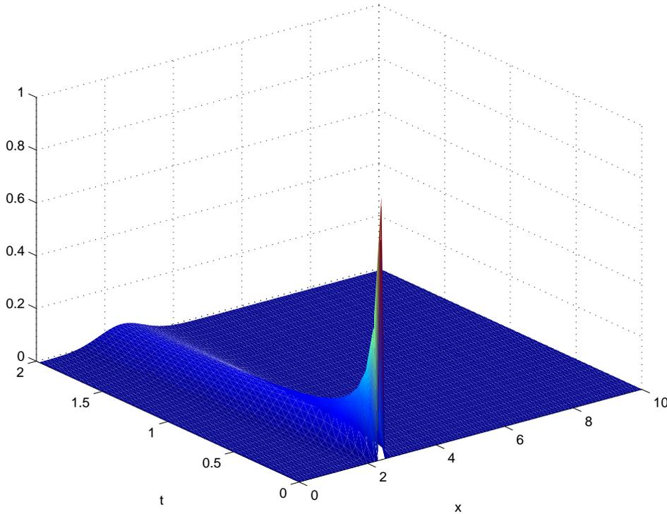
Figure 5: Numerical solutions for the solution of Jeffrey's equation obtained using the splitting method (25), (26) ( $\frac{k_i}{\gamma} = 0.1, i = 1, 2, \tau = 1, h = 0.1, \Delta t = 0.06$ ).
