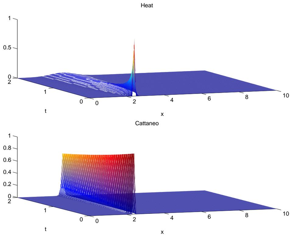
Figure 1: Solutions of the heat equation and Cattaneo's equation with a Dirac delta initial condition.
