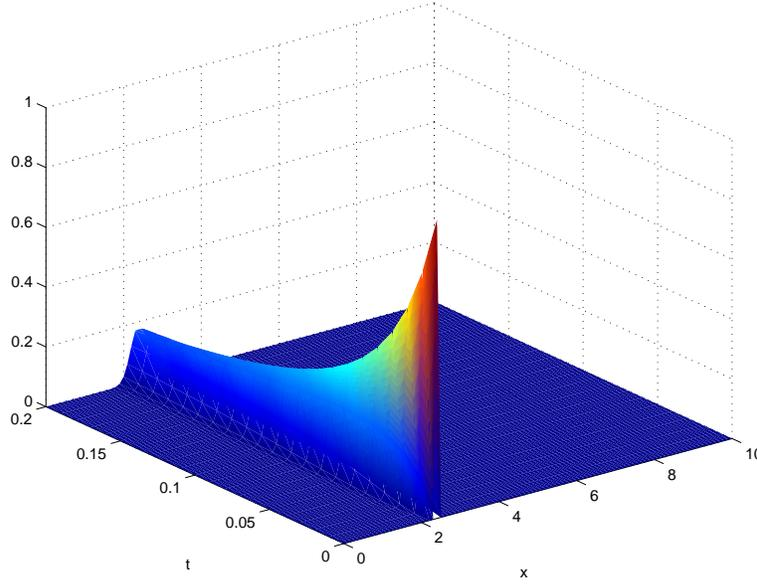
Figure 3: Numerical solution of Jeffrey's equation obtained using method (15) with  $\frac{k_i}{\gamma} = 0.1$ ,  $\tau = 1$ ,  $h = 0.1$ ,  $\Delta t = 0.03$ .
