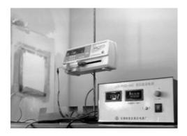
Figure 1 System setup for electrospinning process.
