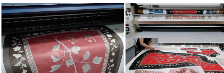
Fig. 10: The process of digital printing
