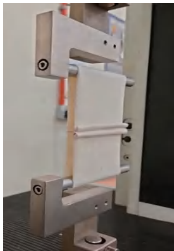
Fig. 2: Looped fabric sample mounted on the looped bar of the tensile machine.
