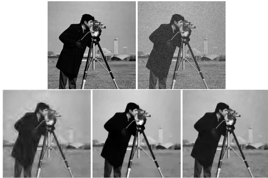
Figure 7: Experiments on Cameraman. Top-left: clean image; top-right: noisy image degraded by Gaussian noise of standard deviation 20, SNR = 9.87 ; bottom-left: wavelet soft-shrinkage with \alpha = 50 , SNR = 11.89 ; bottom-middle: ROF, SNR = 13.61 ; bottom-right: new model with \alpha = 50 , \beta = 60 , SNR = 15.73 .
