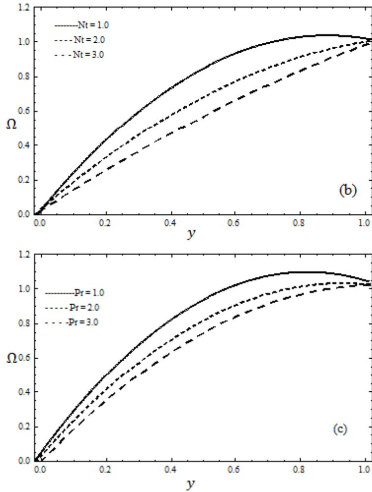
Fig. 3 Concentration  $\Omega$  versus  $y$  when  $t = 0.1, x = 0.2, \varphi = 0.6, Q=0.25, \lambda =10, k =0.1, a_{20}=2.0$ ; (a)  $Nt=0.4, Pr=6.9$ . (b)  $Pr=6.9, Nb=0.4$ . (c)  $Nt=0.4, Nb=0.4$ .
