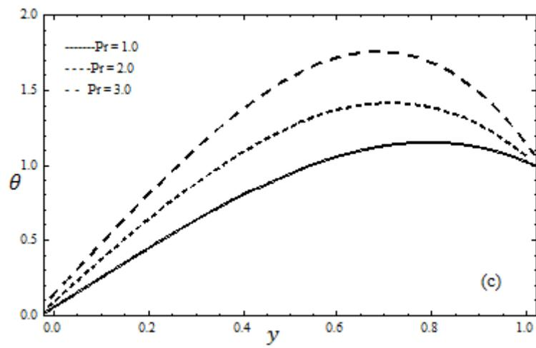
Fig. 2 Temperature  $\theta$  versus  $y$  when  $t = 0.1$ ,  $x = 0.2$ ,  $\varphi = 0.6$ ,  $Q=0.25$ ,  $\lambda = 10$ ,  $k = 0.1$ ,  $a_{20}=2.0$ ; (a) $Nt=0.4$ ,  $Pr=6.9$ . (b) $Pr=6.9$ ,  $Nb=0.4$ . (c)  $Nt=0.4$ ,  $Nb=0.4$ .
