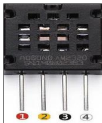
Fig.22. Physical shape and specifications of A2320 sensor along with sample measurements.
