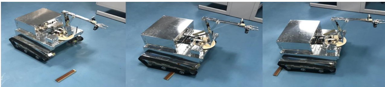
Fig.35. Climbing small obstacles test.
