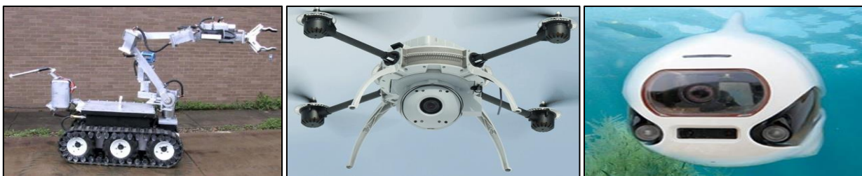
Fig.1. Illustration Examples of UGV, UAV, UUV respectively
