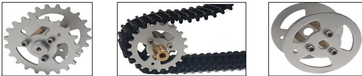
Fig.5. (a) 5 cm diameter tank driving wheel (b) Implementation of driving wheel & continuous track (c) Supporting wheel
