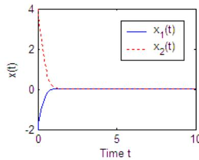
Fig. 6 The state trajectories with  $x(0) = [-2 \ 4]^T$
