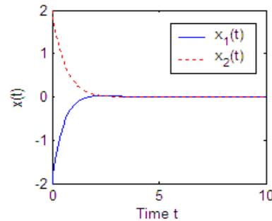
Fig. 8 The state trajectories with  $x(0) = [-2 \quad 2]^T$
