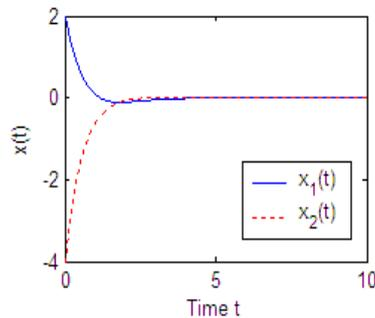
Fig. 7 The state trajectories with  $x(0) = [2 \quad -4]^T$
