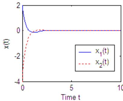
Fig. 3: The state trajectories with  $x(0) = [2 \ -4]^T$
