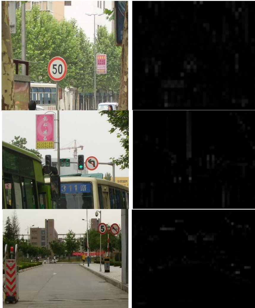
(a) The original images (b)The corresponding saliency maps Figure 1.The saliency maps using our method
