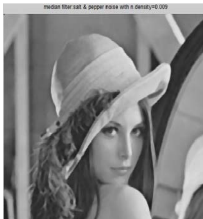
Fig. 18: De-noising by Median Filter for Salt & Pepper noise with noise density=0.009
