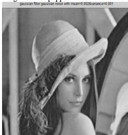
Fig. 5: De-noising by Gaussian Filter for Gaussian noise with mean= 0.002 and variance = 0.001
