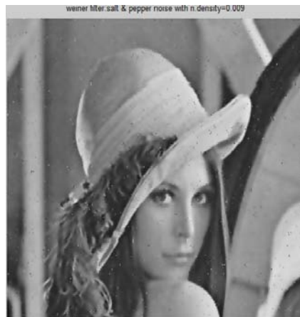
Fig. 15: De-noising by Wiener Filter for Salt & Pepper noise with noise density=0.009
