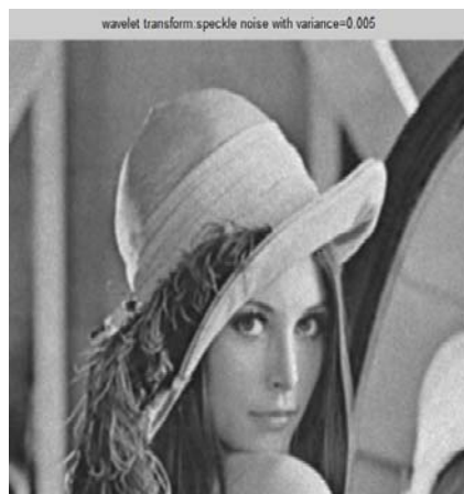
Fig. 14: De-noising by Wavelet Transform for Speckle noise with variance=0.005
