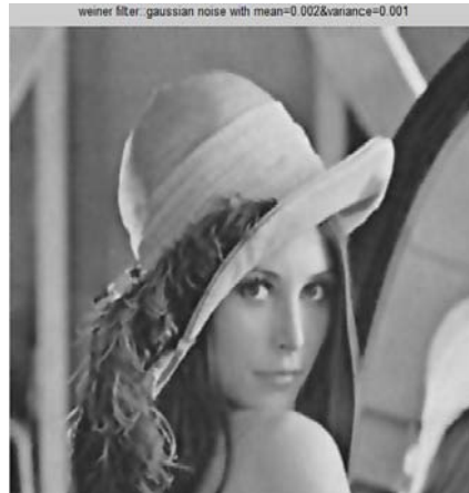
Fig. 7: De-noising by Wiener Filter for Gaussian noise with mean= 0.002 and variance=0.001
