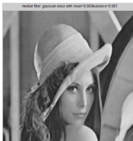
Fig .8: De-noising by Median filter for Gaussian noise with mean=0.002 and variance=0.001
