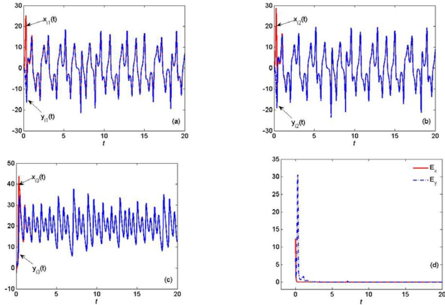
Fig.1. The state of the variables (a)  $x_{i1}$  (red line) and  $y_{i1}$  (blue dot line) (b)  $x_{i2}$  (red line) and  $y_{i2}$  (blue dot line) (c)  $x_{i3}$  (red line) and  $y_{i3}$  (blue dot line); (d) the inner synchronization error of the drive network  $E_x$  and that of the response network  $E_y$ , respectively.
