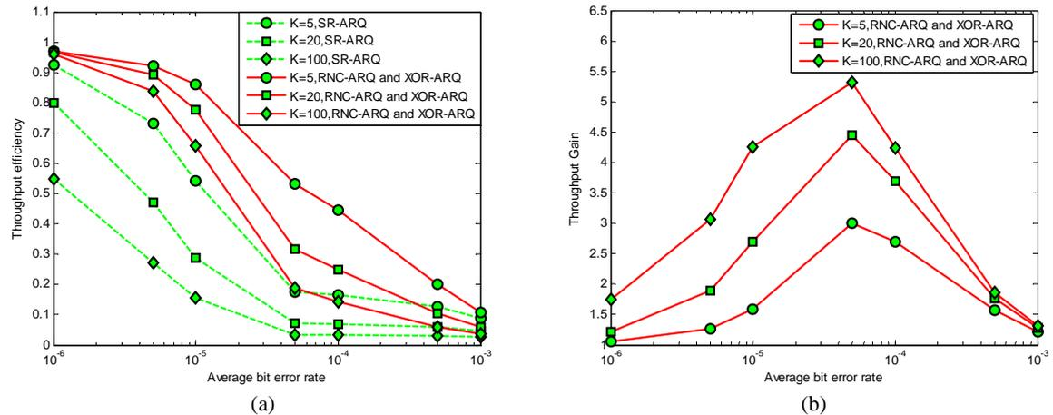
Fig.7 (a) Throughput efficiency of three schemes with  $\bar{b} = 10, P_1 = 0.1$ , and various values of  $K$
