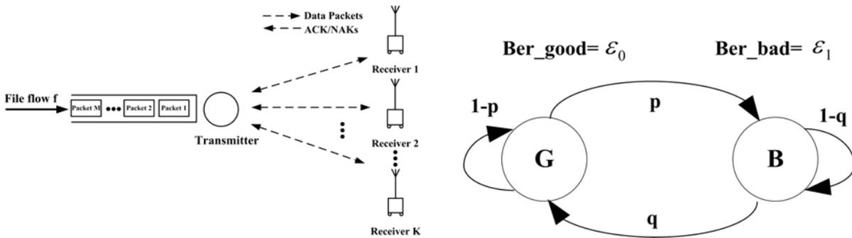
Fig.1 Wireless broadcast system model. Fig.2 Burst error channel modeled by a two-state Markov chain
