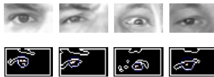
Fig. 5. Using the Hough transform on eye contour image.
