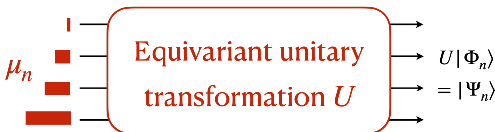
Figure 1.1: Architecture of the variational density matrix representation (1.3) of the present approach. A discrete probabilistic model \mu_n parametrizes the Boltzmann distribution of a many-body basis set |\Psi_n\rangle . We construct |\Psi_n\rangle by applying a parametrized unitary transformation to a reference basis |\Phi_n\rangle . The unitary transformation corresponds to a permutation equivariant many-body coordinate transformation implemented as a flow of fermion coordinates.
