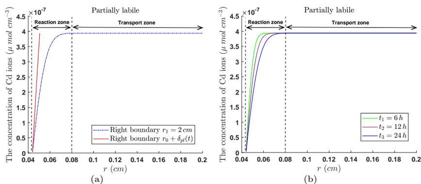
**Figure 6.**  $\text{Cd}^{2+}$  concentration distribution in soil when  $ml$  is partially labile: (a) comparison results of model (2.9)-(2.14) under kinds of right boundaries in one day; (b) the concentration profiles of the model (2.9)-(2.14) along radial distance as  $r_1 = 2$  cm at different times
