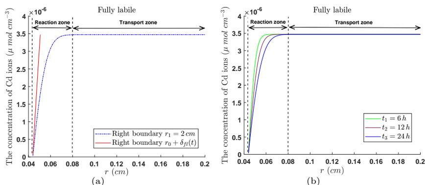
**Figure 5.**  $\text{Cd}^{2+}$  concentration distribution in soil when  $ml$  is fully labile: (a) comparison results of model (2.5)-(2.8) under kinds of right boundaries in one day; (b) the concentration profiles of the model (2.5)-(2.8) along radial distance as  $r_1 = 2$  cm at different times
