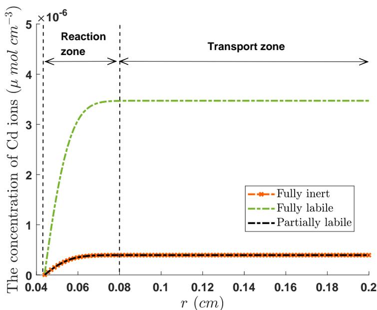
Figure 7. The Cd<sup>2+</sup> concentration as the right boundary  $r_1 = 2 \text{ cm}$  in one day.
