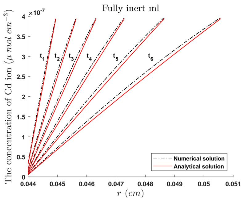
**Figure 1.** The numerical and steady analytical solutions of  $\text{Cd}^{2+}$  concentration in  $t_1 = 0.5$  hours,  $t_2 = 1.5$  hours,  $t_3 = 3$  hours,  $t_4 = 6$  hours,  $t_5 = 12$  hours and  $t_6 = 1$  day, when the complex is fully inert
