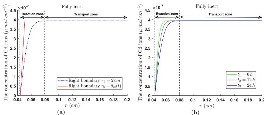
**Figure 4.**  $\text{Cd}^{2+}$  concentration distribution in soil when  $ml$  is fully inert: (a) comparison results of model (2.2)-(2.4) under kinds of right boundaries in one day; (b) the concentration profiles of models (2.2)-(2.4) along radial distance as  $r_1 = 2 \text{ cm}$  at different times
