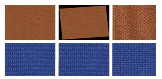
Fig. 5: The skew correction results of knitted fabrics
