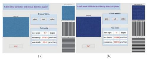
Fig. 7: Fabric skew correction and density detection system: (a) Test result of plain woven fabric; (b) Test result of knitted fabric
