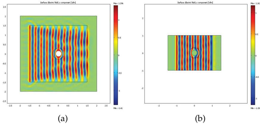
Figure 2: The real part of the electric-field phasor obtained for the cylinder cloak: (a) A big structure; (b) A small structure.
