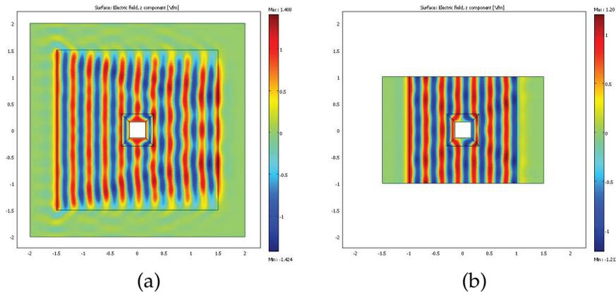
Figure 3: The real part of the electric-field phasor obtained for the square cloak: (a) A big structure; (b) A small structure.
