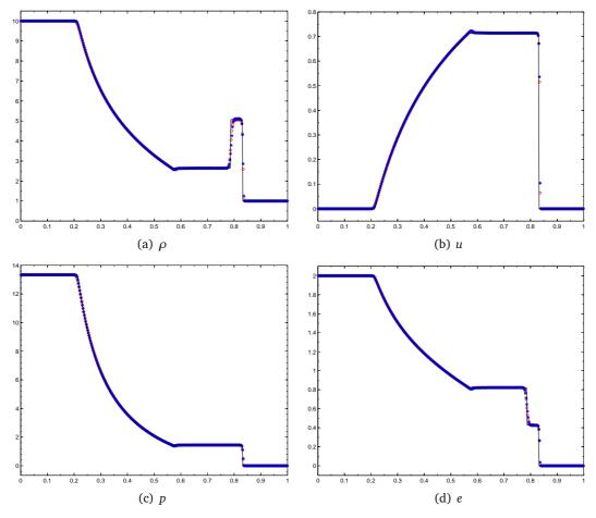
Figure 5: Example 4.2: density  $\rho$ , the velocity u, the pressure p and internal energy e at t = 0.4 with 400 uniform cells.
