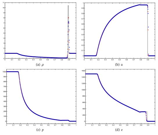
Figure 6: Example 4.3: density  $\rho$ , the velocity u, the pressure p and internal energy e at t = 0.4 with 400 uniform cells.
