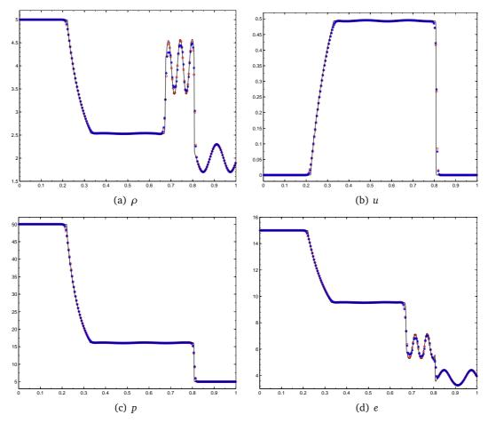
Figure 8: Example 4.5: density  $\rho$  (and its close-up), the velocity u, and the pressure p at t = 0.35 with 400 uniform cells.
