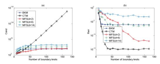
Figure 3: (a) The condition number of the interpolation matrices and (b) the convergent rates of Example 1 by the present CTM, BKM and MFS with different fictitious boundary parameters (d = 2, 8, 14).
