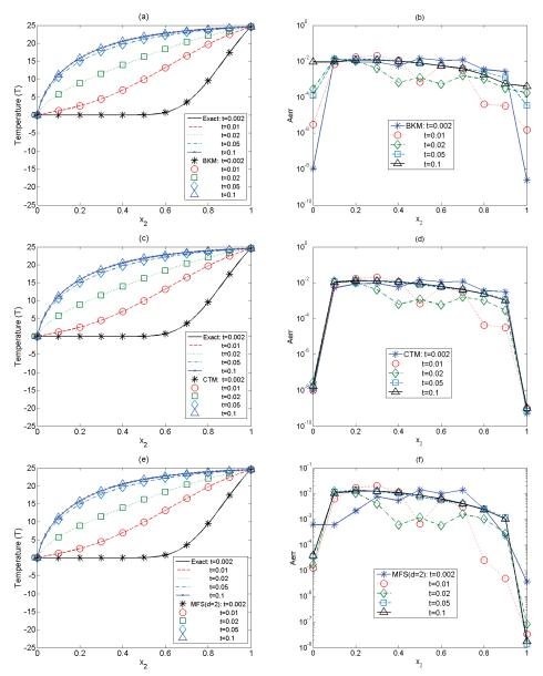
Figure 9: Temperature profile of Example 3 along with  $x_2$ -axis at different time levels by the present (a) BKM, (c) CTM and (e) MFS (d = 2); The corresponding error variation by the present (b) BKM, (d) CTM and (f) MFS (d = 2).
