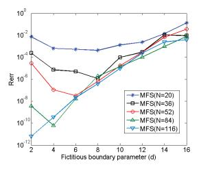
Figure 2: Effect of fictitious boundary parameter d on numerical accuracy in the MFS.
