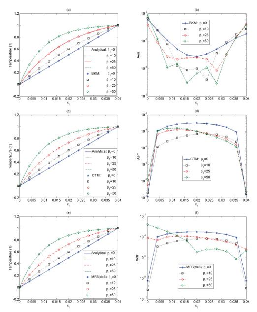
Figure 7: Temperature variation along with  $x_1$ -axis for functionally graded finite strip under steady state loading conditions in Example 2 by the present (a) BKM, (c) CTM and (e) MFS (d = 8); The corresponding error variation by the present (b) BKM, (d) CTM and (f) MFS (d = 8).
