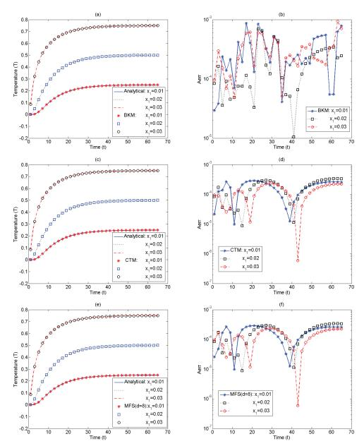
Figure 5: Temperature variation in a finite strip with respect to time (t) at three different locations of Example 2 with  $\beta_1 = 0$  by the present (a) BKM, (c) CTM and (e) MFS (d = 8); The corresponding error variation by the present (b) BKM, (d) CTM and (f) MFS (d = 8).
