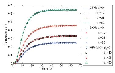
Figure 6: Temperature variation of functionally graded finite strip against time at point (0.01, 0.02) by the present CTM, BKM and MFS (d = 3).
