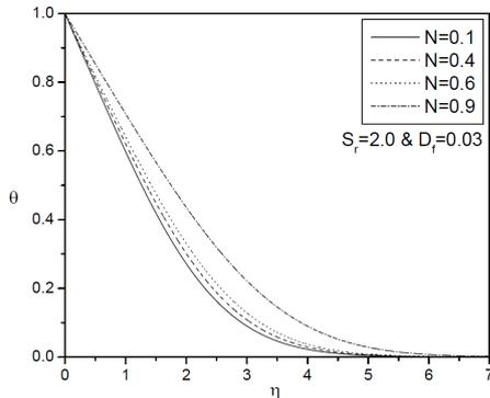
Figure 4: Temperature profiles for various values of  $N$ .
