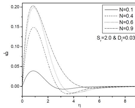
Figure 3: Microrotation profiles for various values of  $N$ .
