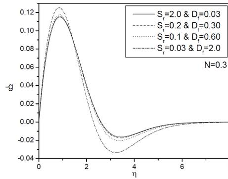
Figure 7: Microrotation profiles for various values of  $S_r$  and  $D_f$ .
