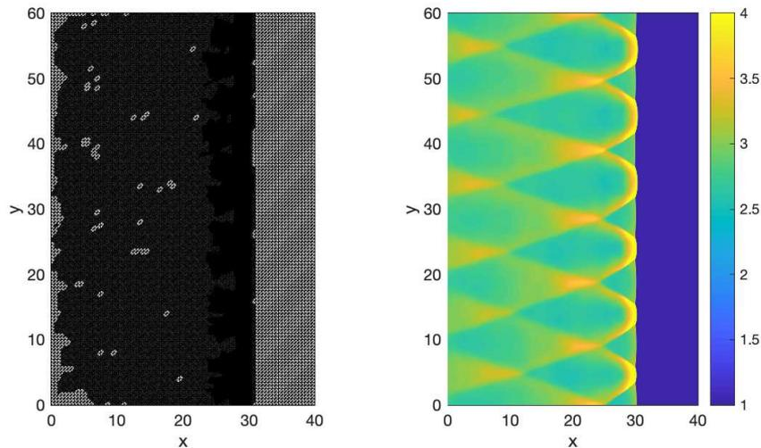
Figure 11: The mesh grids (left), as well as the pressure distribution (right), obtained from simulations on adaptive refined meshes(47926 cells) at  $t \approx 70$ , with the width of the domain 60.
