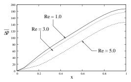
Figure 13: Distribution of mean pressure drop  $\Delta \bar{p}$  with x (k = 0.1,  $\alpha = 1.5$ ).
