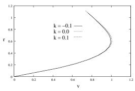
Figure 8: Distribution of transverse velocity (v) with y (Re = 1.0,  $\alpha = 1.0$ , x = 0.2).
