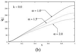
Figure 11: (a) Distribution of mean pressure drop  $\Delta \bar{p}$  with x (k = 0.1, Re = 1.0); (b) Distribution of mean pressure drop  $\Delta \bar{p}$  with x (k = 0.0, Re = 1.0); (c) Distribution of mean pressure drop  $\Delta \bar{p}$  with x (k = -0.1, Re = 1.0).
