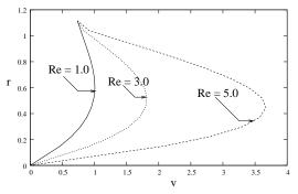
Figure 9: Distribution of transverse velocity (v) with y (k = 0.1,  $\alpha = 1.0$ , x = 0.2).
