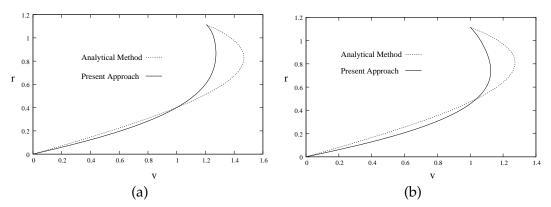
Figure 6: (a) Comparison of transverse velocity between Analytical method and numerical approach ( $\alpha = 2.0$ ); (b) Comparison of transverse velocity for between Analytical method and numerical approach ( $\alpha = 1.5$ ).
