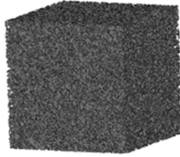
Figure 3: A representative porous structure applied for the underresolved regions in the multiscale simulation in Section 4.
