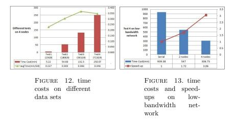
In order to evaluate the performance of the prototype on WAN, we migrate the prototype to a low-speed network on which all computation nodes share 10Mbps bandwidth. Benchmark result on test case 4 is shown in figure 13. Unsurprisingly, the parallel processing efficiency is reduced for about 18% because it costs more time for transferring commands and messages on WAN. But, speed-up over 3 on
