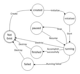
FIGURE 8. states of an instance in a life-cycle
