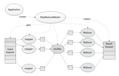
FIGURE 6. MapReduce based on Robinia
