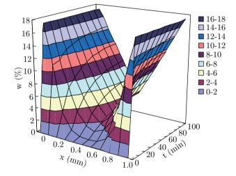
Fig. 6: Humidity distribution in the fabric
