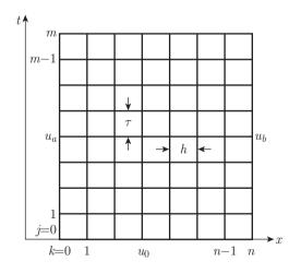
Fig. 3: Finite difference grid
