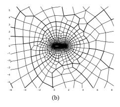
Figure 2: Example 2: (a) Mesh 5 partitioned into 500 regions using METIS; (b) Zoom of (a); (c) Further zoom of (a).
