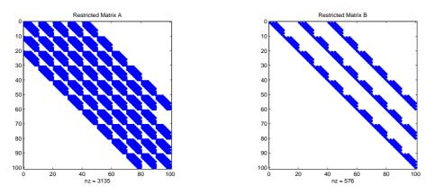
Figure 2: Non-zero (nz) elements of 2-D pre-multiplied restricted Galerkin operator A (left) and quasiinverse B (right) for the 2-D Helmholtz problem with 12 \* 12 Chebyshev grids.
