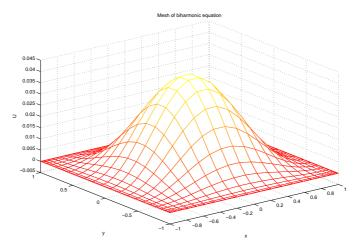
Figure 5: Numerical solution of the 2-D biharmonic problem with 24 \* 24 Chebyshev grids.
