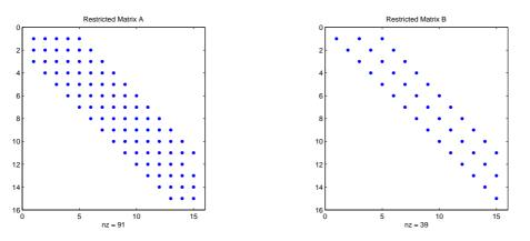
Figure 1: Non-zero (nz) elements of 1-D pre-multiplied restricted Galerkin operator A (left) and quasiinverse B (right) from Eq. (3.17) with 17 Chebyshev grids.
