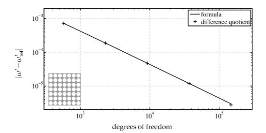
Figure 4: Convergence of the error of the group velocity formula (solid line) and the first order difference quotient (markers) when increasing the grid refinement of a finite element computation with polynomial degree one. The reference solution is computed with polynomial degree 20.
