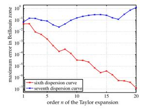
Figure 6: Maximum error of the Taylor expansion of the sixth (red) and seventh (blue) dispersion curve of the band structure presented in Figure 5 in dependence on the order n of the Taylor expansion. The maximum error is evaluated on an equidistant grid of 40 values of  $k \in \hat{B}$ .
