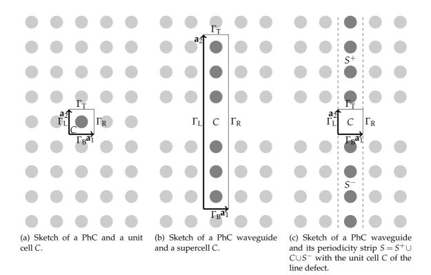
Figure 1: Sketches of the computational domains C, *i.e.* of the unit cell of a PhC (a), a supercell of a PhC waveguide (b), and a unit cell of the line defect of a PhC waveguide (c) with their boundaries  $\Gamma_L$ ,  $\Gamma_R$ ,  $\Gamma_T$  and  $\Gamma_B$ , and periodicity vectors  $\mathbf{a}_1$  and  $\mathbf{a}_2$ .
