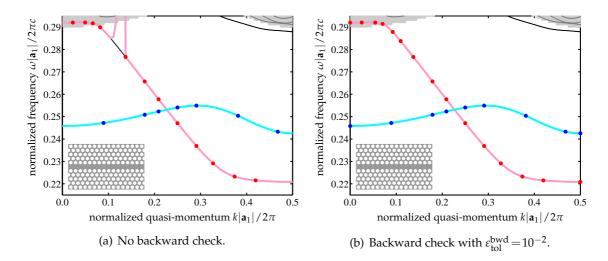
Figure 9: Adaptive Taylor scheme of order n = 10 applied to dispersion curves of the hexagonal W1 PhC waveguide. The error tolerance of the step size computation is  $\varepsilon_{tol}^{step} = 10^{-4}$  and the start value of the iteration is set to  $k^{(0)} = \pi/(2|\mathbf{a}_1|)$ .
