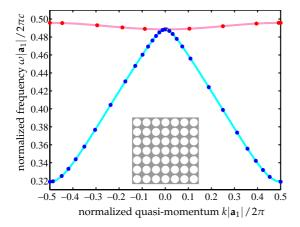
Figure 14: Adaptive Taylor scheme of order n=3 with backward check of tolerance  $\varepsilon_{\rm tol}^{\rm bwd}=10^{-2}$  applied to the second and third dispersion curves of Example 2.1. The start value of the scheme is set to  $k^{(0)}=0.25\cdot 2\pi/|{\bf a}_1|$ .
