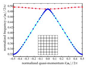
Figure 15: Adaptive Taylor scheme of order n=2 with backward check of tolerance  $\varepsilon_{\rm tol}^{\rm bwd} = 10^{-2}$  and second order mini-stop band check of tolerance  $\varepsilon_{\rm tol}^{\rm msb} = 10^{-2}$  applied to the second and third dispersion curves of Example 2.1. The start value of the scheme is set to  $k^{(0)} = 0.25 \cdot 2\pi / |\mathbf{a}_1|$ .
