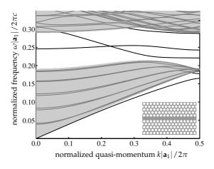
Figure 8: Band structure (black lines) of the TE mode in a hexagonal W1 PhC waveguide. The holes of relative radius 0.31 have permittivity  $\varepsilon = 1$  and are surrounded by dielectric material of permittivity  $\varepsilon = 11.4$ . The computation was performed using the supercell method with five periodicity cells on top and bottom. The frequencies at which propagating PhC modes exist are shaded in grey while blank areas represent the band gaps.
