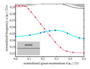
Figure 10: Adaptive Taylor scheme of order n = 10 with backward check of tolerance  $\varepsilon_{tol}^{bwd} = 10^{-2}$  applied to dispersion curves of the perturbed W1 PhC waveguide of hexagonal lattice (upper PhC shifted by  $10^{-4}|\mathbf{a}_1|$  to the left). The error tolerance of the step size computation is  $\varepsilon_{tol}^{step} = 10^{-4}$  and the start value of the iteration is set to  $k^{(0)} = \pi/(2|\mathbf{a}_1|)$ .
